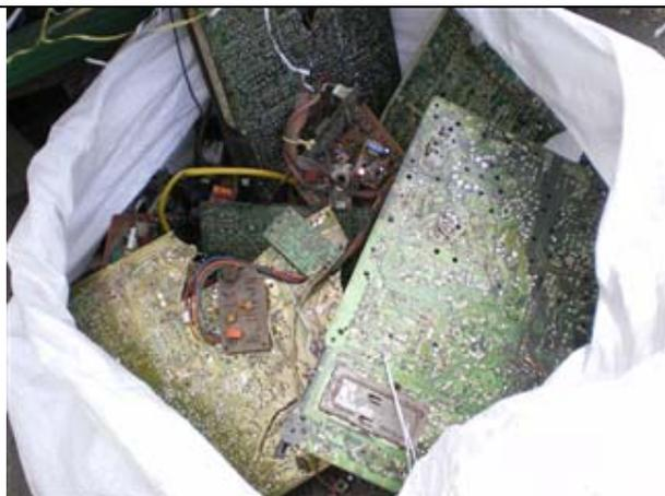
Printed circuit boards from e-waste are segregated manually for further recycling mainly non-ferrous metal recovery in other location including abroad.
