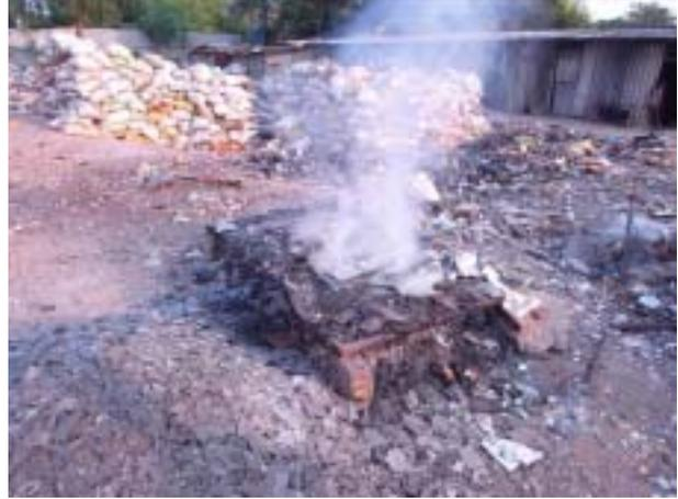
Glasses with wires (ex. windows) are crushed into pieces to separate from wires. Glasses with films are burned to make the film melt.
