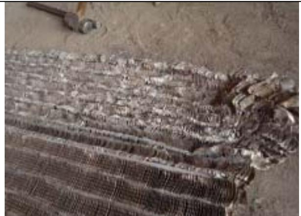
Aluminum taken by AC. They are separated from steel pipes, and flattened, and broken into pieces before sold to recyclers.
