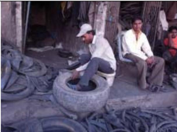
Tires are cut to be able to store more tires in one limited space. Although separated, all parts of a tire will be turned into fuel.
