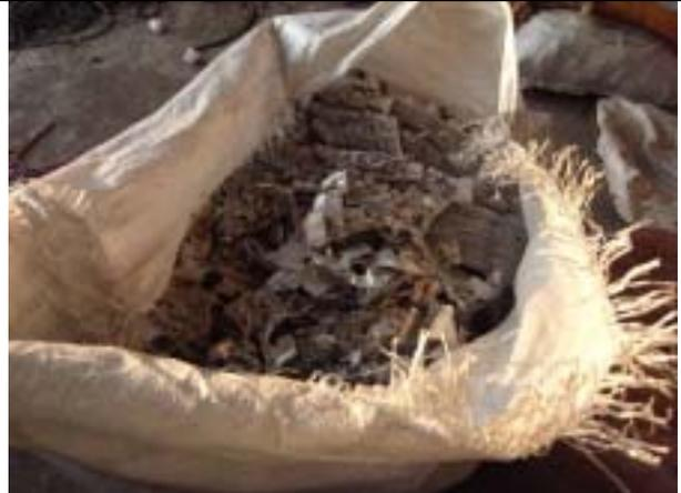
Aluminum broken into pieces. There will be 10% reduction in weight after processing and cleaning.
